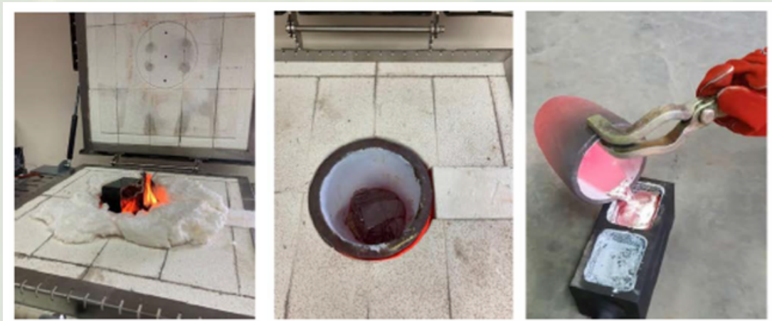
Figure.2 Remelting and casting process of aluminum after thermal pre-treatment
