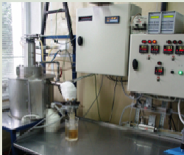
Figure.3 Apparatus for cross formation tests
