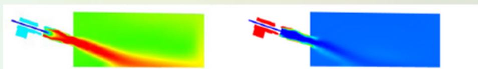
Figure.1 Temperature and oxygen profile for one burner
