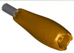
*Figure.1* Flame modelization of new burner
